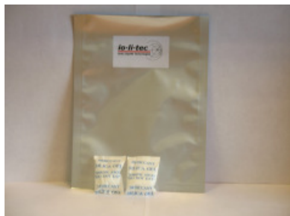
Figure 3. Aluminium composite bags and silica drying pads used by IoLiTec
