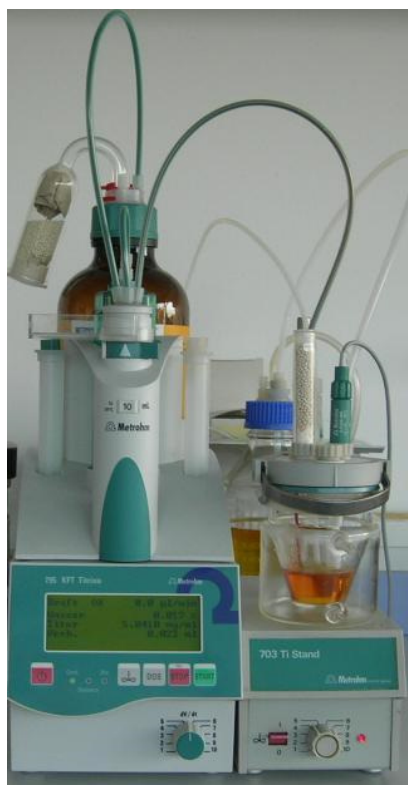
Picture 2. Karl-Fischer-Titration for the determination of water content.
